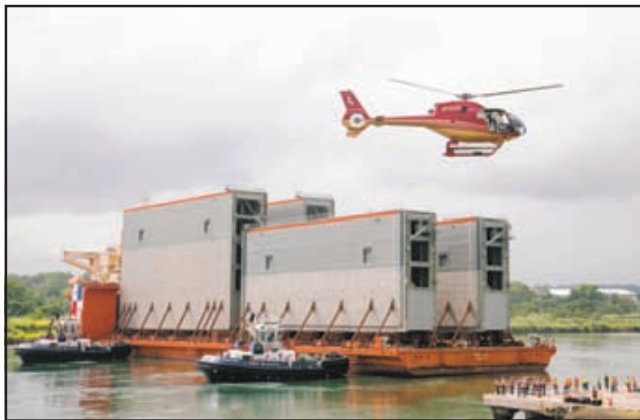
A ship arrives with new rolling gates for the Panama Canal's third set of locks for the canal's expansion project at Limon Bay, Gatun, Panama, Tuesday, June 10, 2014.
