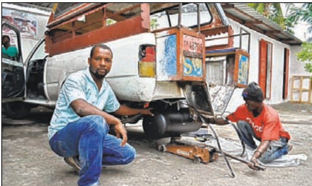
A new step: Propane tank being installed under a taxi for use. This conversion from gas dependency will reduce pollution caused by gas-running vehicles. (right) Jean Conille, founder of Autogaz Haiti.
